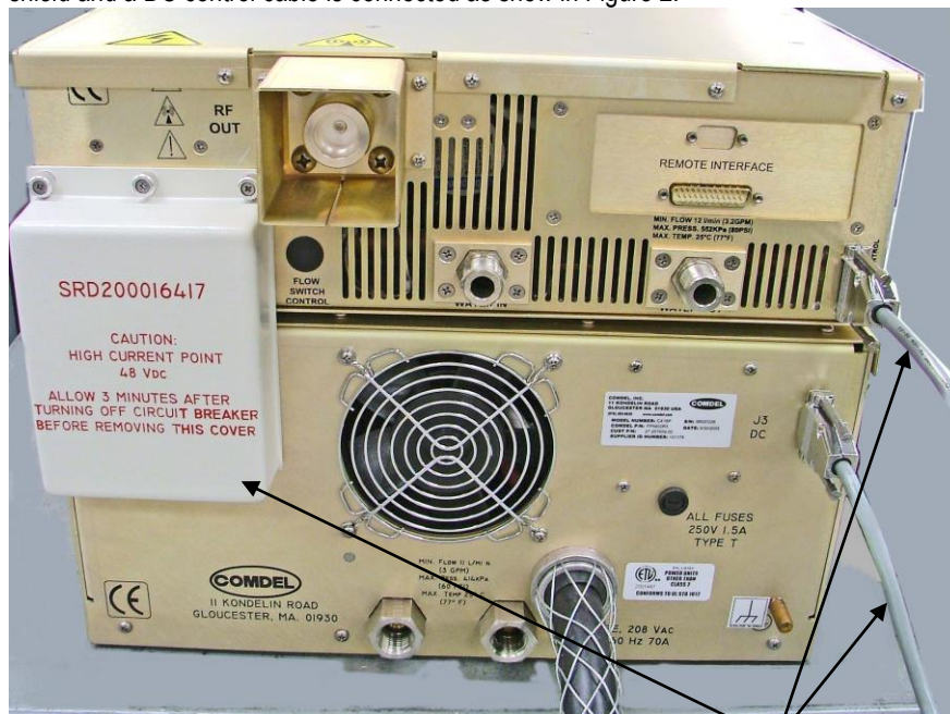
Figure 2. The DC bus safety cover and the DC control cable installed. (NOTE: Picture of bottom DC section shows alternate 8.75" tall linear DC supply. Actual FP6810Rx switching DC supply is 5.25" tall)
